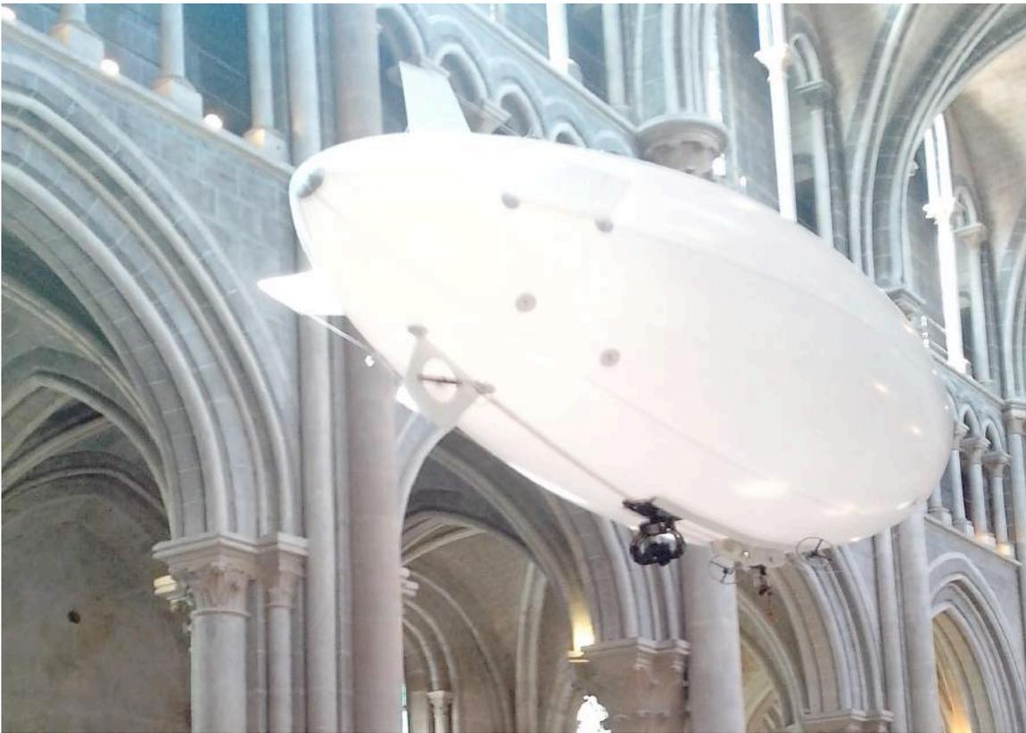
Blimps have higher payload than multicopters, they fly longer and have less vibrations.
